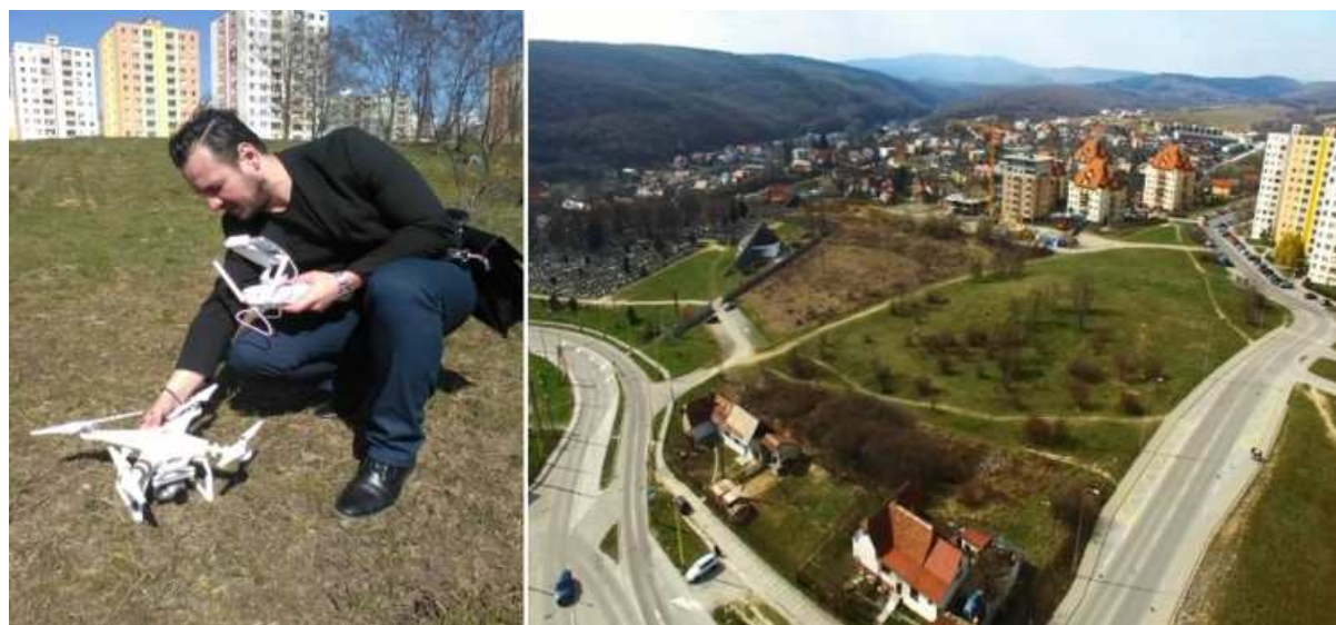
1: Photoshooting the place of a future construction site with a drone for integration into a virtual environment
